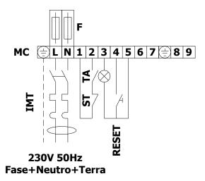
Electrical connection diagram (version with function changeover switch):
