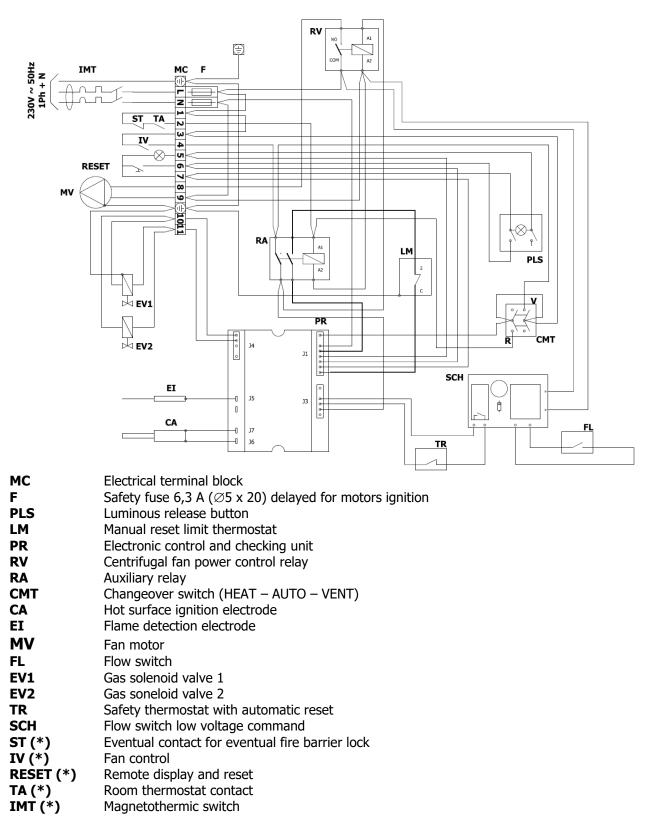
(\*) Not included in the delivery, it should be installed by the customer or the fitter.
