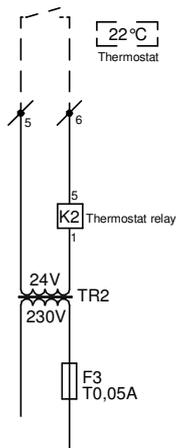
Every heater has to be switched by a **separate** low voltage ON/OFF contact in the control room
