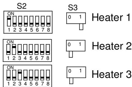
Change the settings from the switches on the control unit in the heater.
