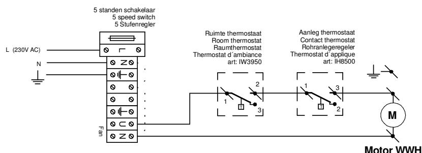
5-step switch with contact thermostat
